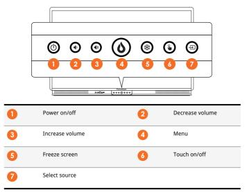
The Power on/off and the Menu button light up to indicate whether the panel is powered on, in standby or in sleep mode.
